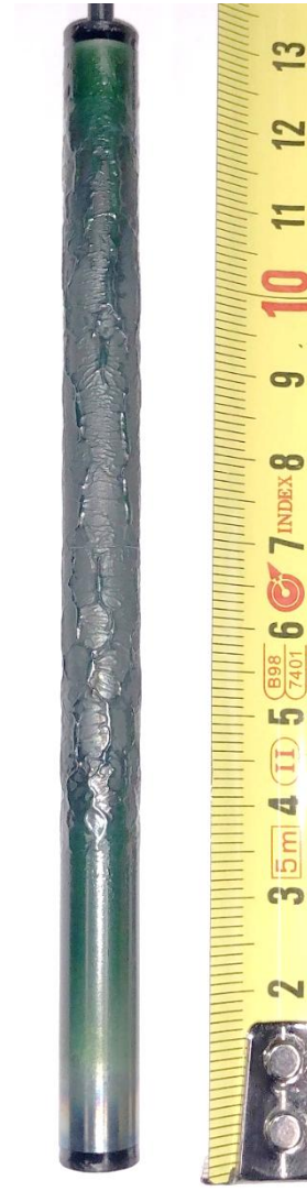
EC1: 8 K/s to T_{\max}=1390\text{ }^{\circ}\text{C} , immediate cooldown
