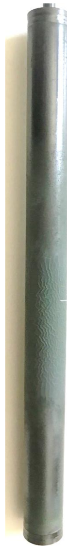
MC-7: 1250 °C during 10 min
