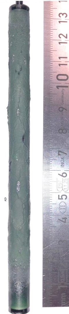
EC3: 8 K/s to T_{\max}=1400\text{ }^{\circ}\text{C} , 240 s 1400\text{ }^{\circ}\text{C} , imm. cooldown
