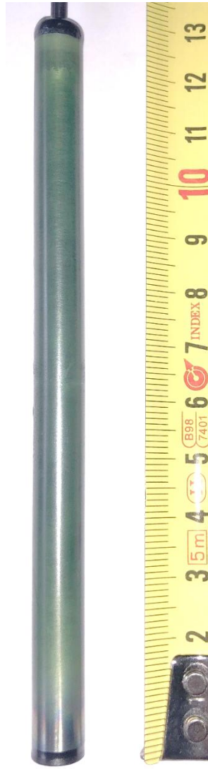
EC4: 5 K/s to 1250\text{ }^{\circ}\text{C} , 5 s 1330\text{ }^{\circ}\text{C} , imm. cooldown
