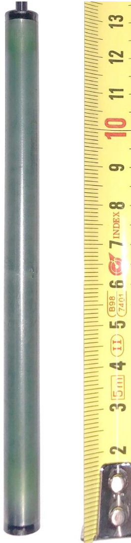
EC2: 5 K/s to T_{\max}=1250\text{ }^{\circ}\text{C} cooldown 2 K/s, quench at 900\text{ }^{\circ}\text{C}
