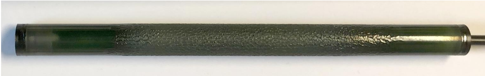
sample MCs-3: transient with 8 K/s, then 1400 °C during 3 s
