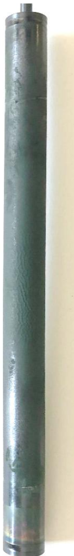
MC-5: 1200 °C during 15 min
