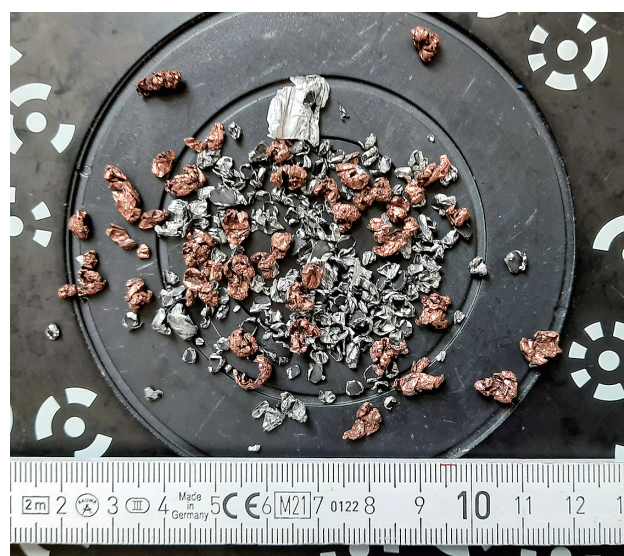
Fig. 2 Particles from the mechanical recycling process of lithium-ion-batteries as explained in (Werner D. et al., 2020), showing particles with non-compact irregular and significantly distributed shape properties.
