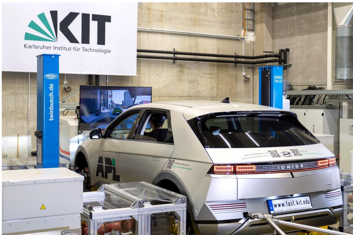
Fig. 1 Powertrain test bench – vehicle-in-the-loop
