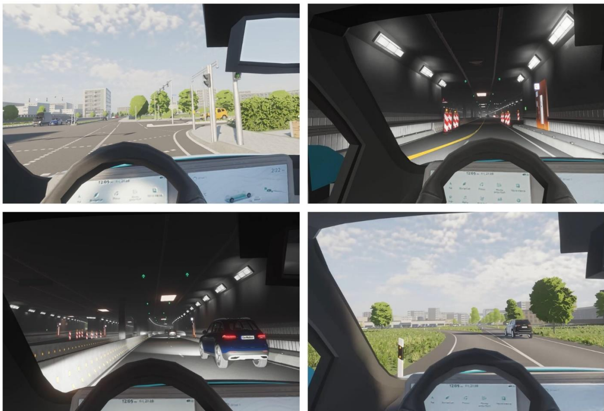
Fig. 6 Possible test cases – Top left: ACC with stop&go function; Top right: construction zones with corresponding takeover situations; Bottom left: challenging lighting condition; Bottom right: handover function for highway driving assist
