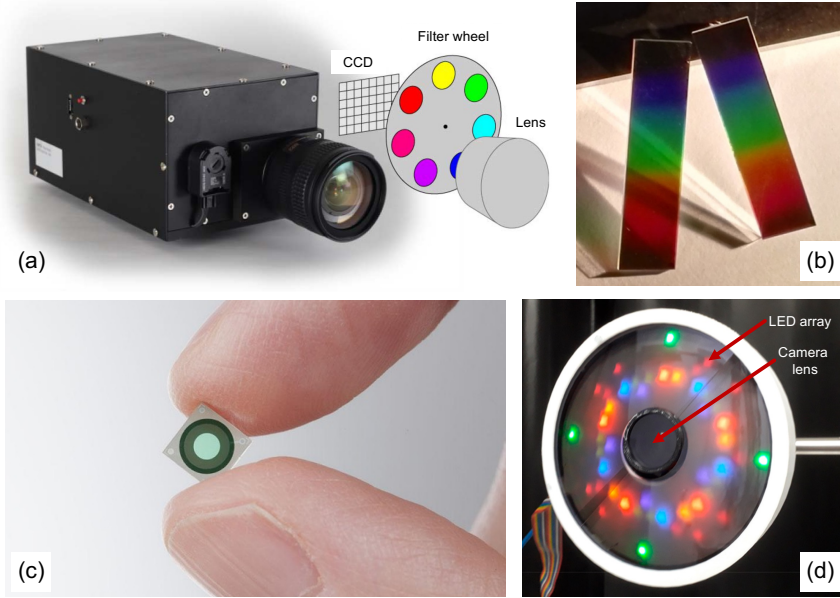
Figure 2.3: Different realizations of the spectral-scan technique with different methods for providing the wavebands sequence: (a) Filter wheel (reproduced from [39] ©2008 IEEE). (b) Linear variable filter (reproduced with permission from [42] ©2019 Optical Society of America). (c) Fabry-Pérot tunable filter (cropped from [52] ©2017 SPIE). (d) LED array (adapted with permission from [51] ©2020 American Chemical Society).
