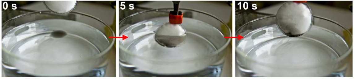
Figure 3.10: Series of images demonstrating the oil absorption of polymeric nanofur. The drop of colored oil (Azolla ZS 32) is selectively absorbed from a bowl of water, thereby cleaning the water. The piece of nanofur was submerged for about 10 s.
