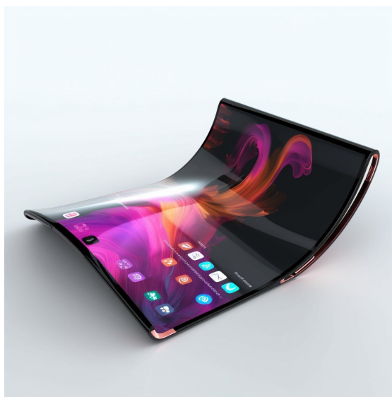
Figure 1.1: Flexible OLED-display. Picture taken from [5]. Copyright 2024 Fluxim AG.
