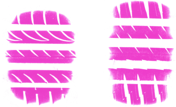
Figure 3.6: Exemplary scans of tire tread visualised with FUJIFILM Corporation Prescale pressure measurement film.
