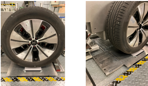
Figure 3.5: Process of creating tire tread patterns with FUJIFILM Corporation Prescale pressure measurement film.
