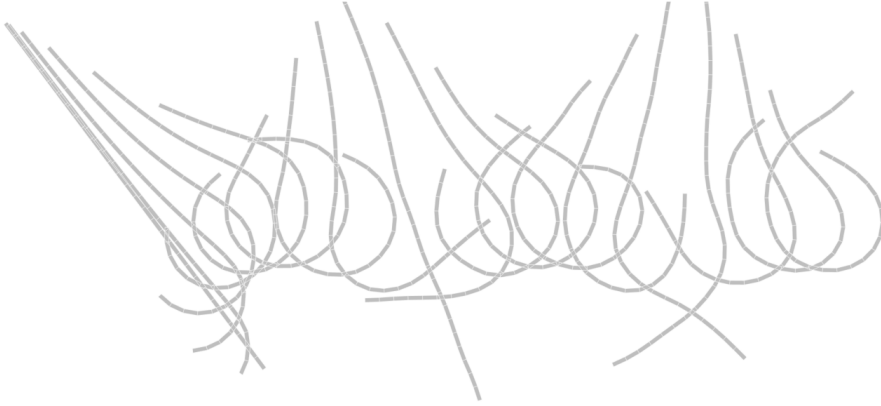
Figure 5.9.: Snapshots of the flight motion of the flying spaghetti (10 LCS3 elements) in increments of \Delta t = 0.5 from t = 0 to t = 10 .
