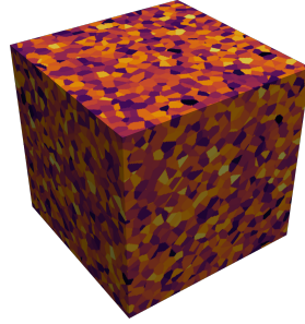
Figure 6.6: Microstructure used for full-field simulations at a resolution of 256^3 . Figure based on Figure 6 of Krause et al. (2024).
