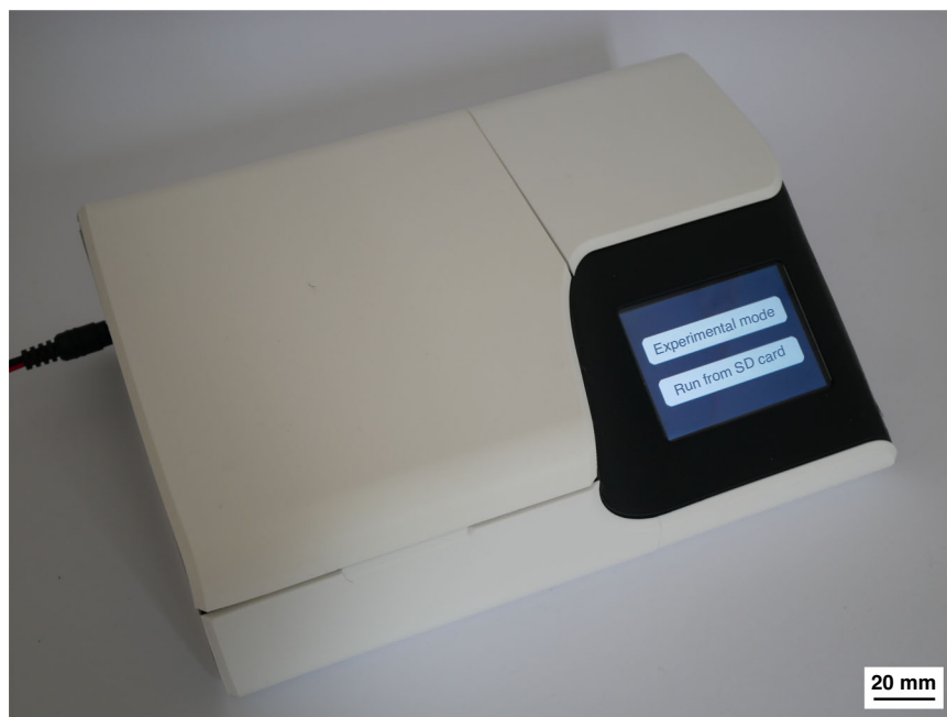
Fig. 9 An image of the open-source device providing the capabilities for DEP and centrifugal microfluidics
