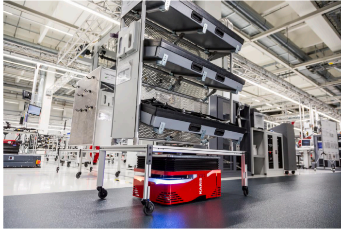
Fig. 4. The KarisPro AMR research prototype delivers a material transport trolley from the picking area to the assembly line.
