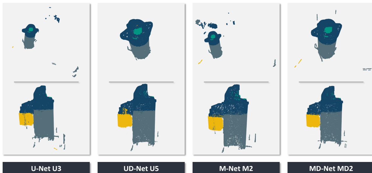
Figure 6.4: Visualization of the reconstructed semantic 3D models based on the segmentation of the image data (RGB and/or depth) using the best model configurations and the acquired point clouds.
