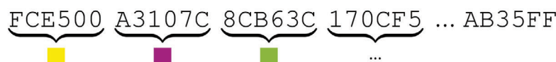
Figure 8. Schematic explanation of hash parsing and conversion into RGB colors saved in C_B (block colors) / C_T (target colors) and light intensity values for four lamps saved in tuple I_T .
