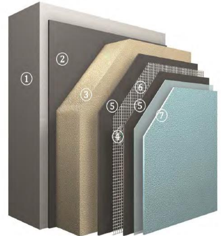
(1) Building envelope, (2) Adhesive mortar, (3) insulating material: EPS, (4) Dowels or rail systems, (5) Reinforcing mortar, (6) Reinforcing mesh, (7) Exterior coating
