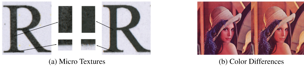
Figure 3.3: (a) Differences of Micro Texture and Edge Roughness printed by HP M553 (left) and HP 4350 (right). (b) Differences of color representations by HP M553 (left) and Ricoh MP305 (right)
