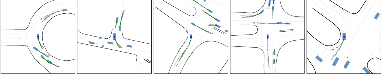
Fig. 4: Qualitative results of joint-StarNet on INTERACTION [7] validation subset. Rectangles indicate vehicles, while squares are pedestrians/bicycles. Gray trajectories are predictions ( m = 3 modes), with the ground truth overlaid in green. The right-most prediction is among the 50 worst individual predictions according to the FDE metric.
