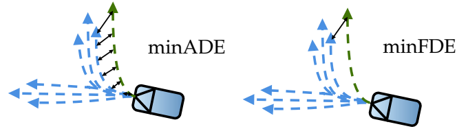
Figure 1.4: Visualization of the minADE and minFDE metrics: the minADE represents the average Euclidean distance between the ground-truth future trajectory (green) and the closest trajectory among the predicted trajectories (blue) for all points. Similarly, minFDE only considers the average distance between the final points.
