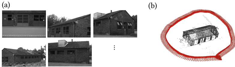
Figure 5.6: Structure-from-Motion experiment, where the camera (red pyramids) was moved around a building. Figure adapted from [Hag22c].
