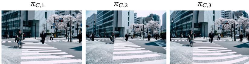
Figure 1.2: Different projection functions will result in different images of the same scene. To extract information on the three-dimensional geometry of the environment, the projection function \pi_C must be known which is achieved through calibration. Image of a street scene in Japan, synthetically transformed to show the impact of different projection models. Original image source: [Pxx18].
