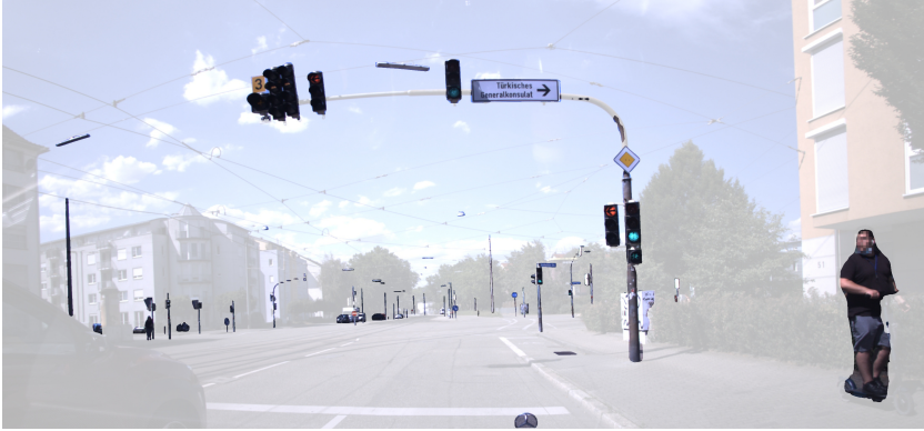
Figure 3.3: Example detections of the DNN used for extracting instance masks on a typical camera image of the 2020 sensor setup. All masks are combined as clear filter while all other pixels are faded out.
