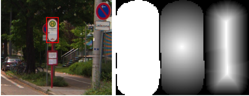
Figure 3.8: Depiction of the proposed schemes to weight lidar points. On the left, a crop of the original image with the detected sign is shown. On the right, the instance mask m with uniform, distance to center point and distance to contour weighting is depicted (from left to right). Brighter color indicates higher weight.
