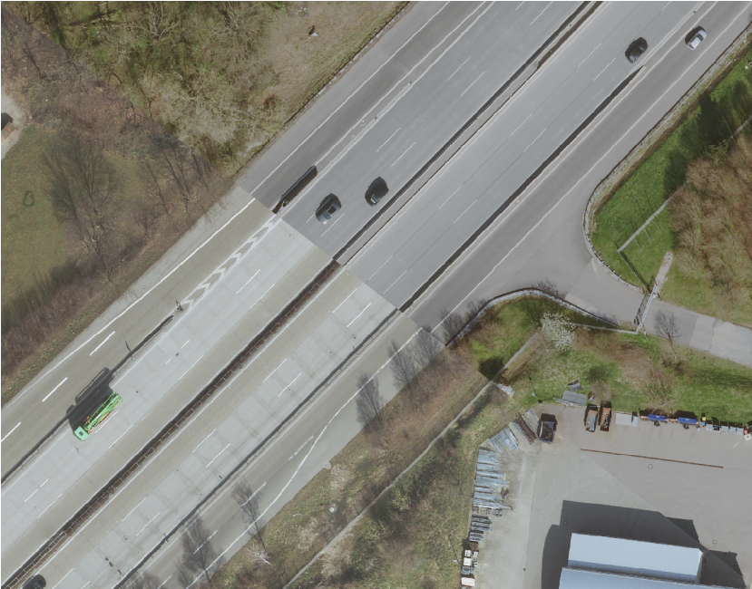
Figure 2.3: Exemplary superimposition of aerial imagery from 2015 (bottom left) and 2017 (top right). While the highway has been changed entirely and even was widened, the unchanged parts next to the highway still allow pixel-accurate geo-referencing. Aerial Imagery: © Stadt Karlsruhe | Liegenschaftsamt
