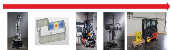
Fig. 1. closed automated chain for decommissioning of NPPs
