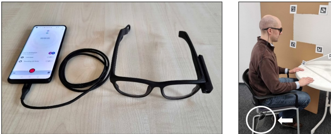
Figure 3.3: Pupil Invisible eye-tracking glasses connected to the Pupil Labs Companion Device (left) and a participant wearing both devices during the first stage (right).
