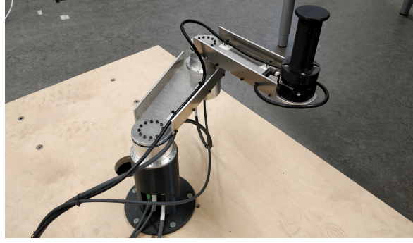
Figure 6.4: The planar SCARA manipulator used for the state estimation experiments on real hardware. Taken from [O2].
