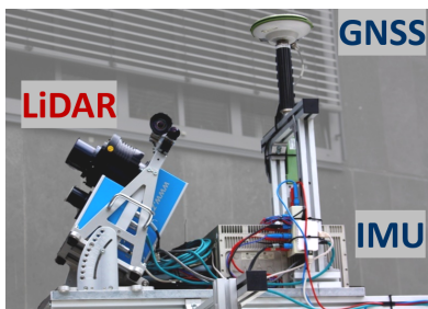
Figure 2. Used MMS. left: Z+F Profiler 9012A profile laser scanner; right: iMAR iNAV-FJI-LSURV IMU and RTK GNSS antenna
