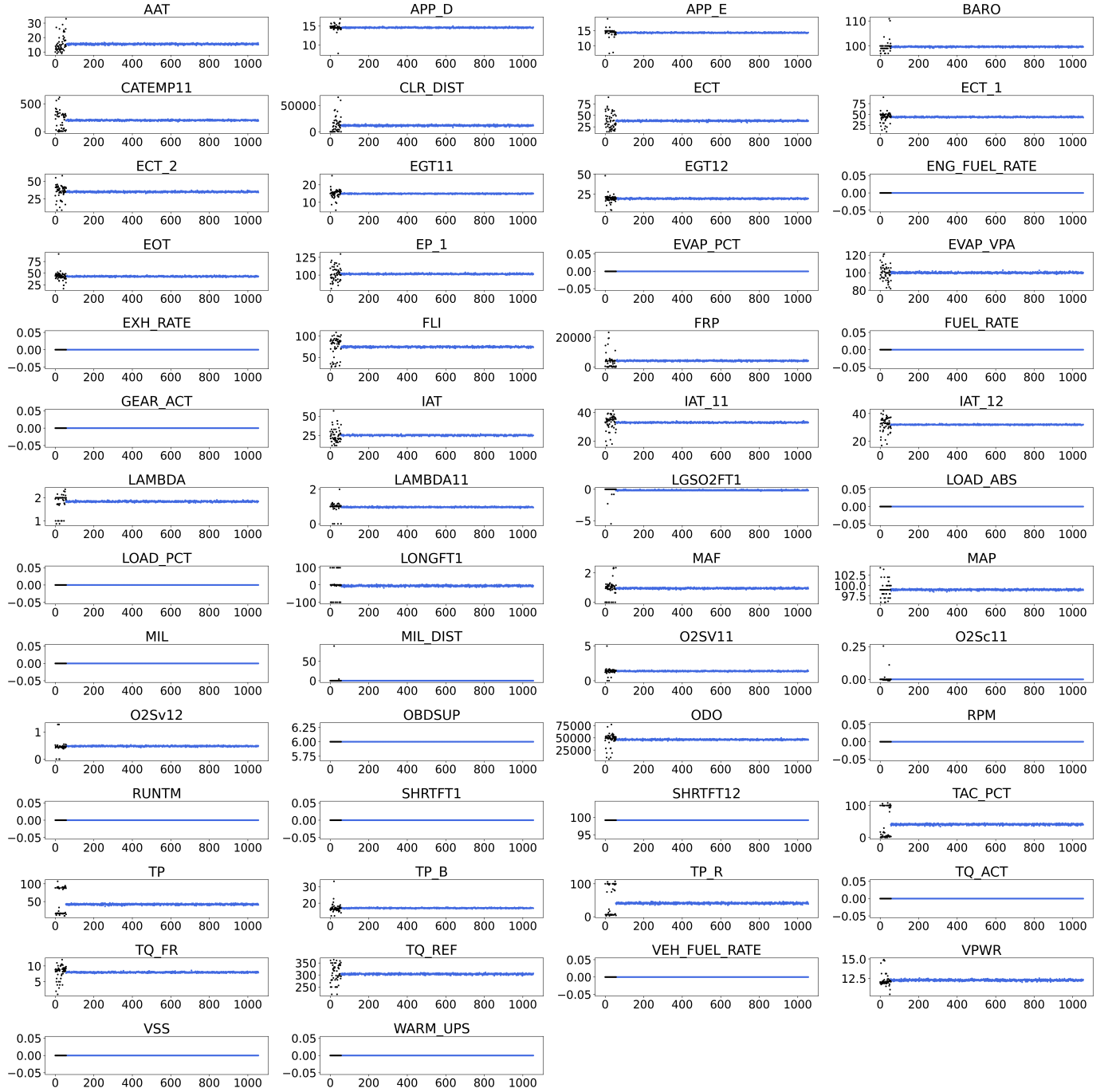
Fig. 6. Comparison of original data (black) and VAE generated data (blue) for the case of 1000 tests and engine off (test 5.6) with all 54 OBD parameters. Each point represents a parameter value from one vehicle.
