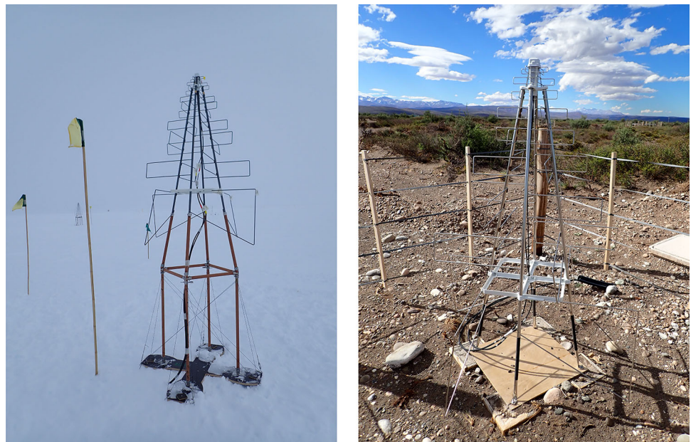
Fig. 5 Photos of SKALA v2 antennas used in prototype stations of the IceCube-Gen2 surface array at IceCube at the South Pole (left) and at the Pierre Auger Observatory in Argentina (right)
