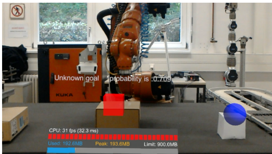
Figure 5.13: The setup for the HIE test with an industrial robot. The goals are predefined as a green cylinder (not visible, left of the image), a red cube and a blue sphere.
