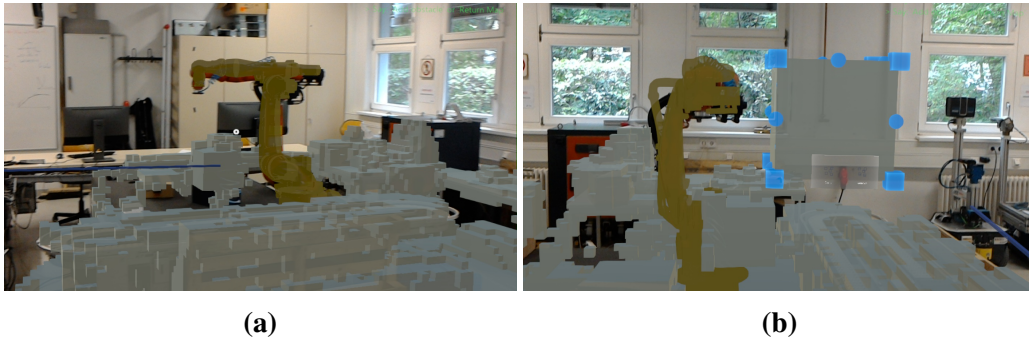
Figure 4.2: (a) Visualisation of the voxel grid representation of the environment in the HoloLens. The individual voxels can be added, moved and removed; (b) Adding safety zones in situ using the HoloLens. Such definition of safety zones are more intuitive and faster than classical input in offline robot programming.
