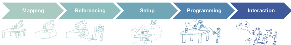
Figure 1.3: The building blocks of our system. Mapping is the first step. It generates a map that is then used to find the robot and calculate coordinate transforms in the referencing block. The coordinate transform and the map are then used to define the robot arm working environment in the setup step. In the programming step various methods may be used to define the desired trajectory of the robot arm. Finally in the interaction step, the human is tracked and their intention estimated for a safer, more intuitive collaboration with robot arms.
