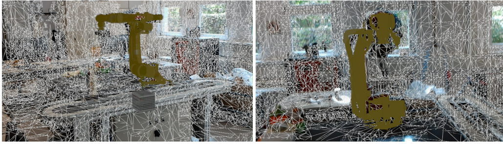
Figure 3.7: The referenced robot as displayed to the user on the HoloLens alongside the seed hologram and the spatial mesh.
