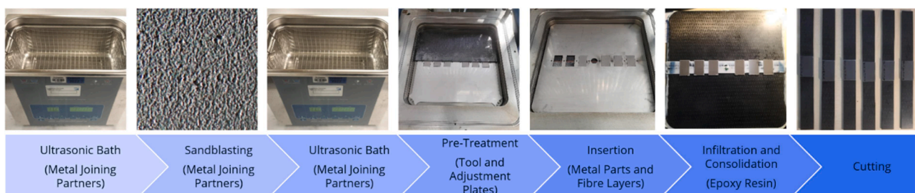
Fig. 1. Manufacturing process of hybrid metal-composite Double-Lap-Shear specimens.
