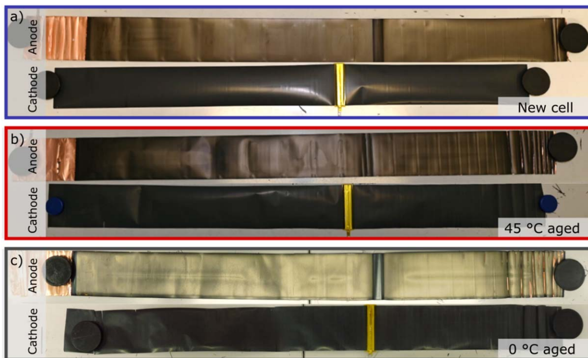
Figure 2. Photographs of unrolled anodes and cathodes from disassembled 18650 cells. (a) new cell, (b) 45 °C aged cell, (c) 0 °C aged cell. The electrode parts that were inside the jelly rolls are on the right hand side.
