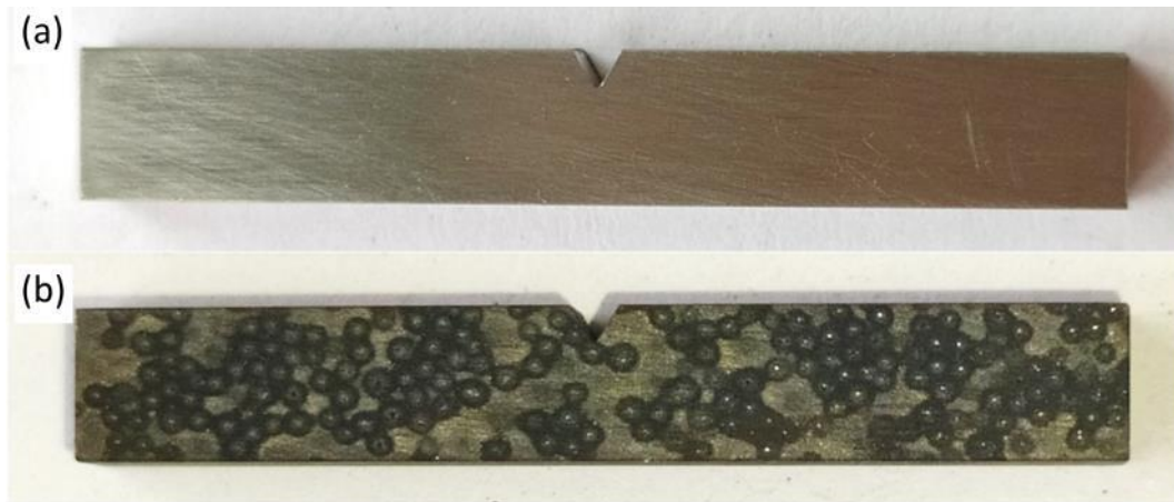
Fig. 4.66. Charpy impact test specimens (a) before and (b) after exposure to the ceramic breeder environment for 64 days
