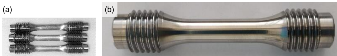
Fig. 3.7 Low-cycle fatigue specimens: (a) sub-sized, (b) standard. Photographs are presented with the preservation of the original size ratio
