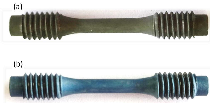
Fig. 4.54. LCF specimens of EUROFER97 for additional experiments: (a) after exposure to Li-ceramics pebbles in vacuum for 64 days, (b) after exposure to a purge gas atmosphere for 64 days [43]
