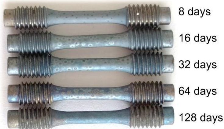
Fig. 4.1. Sub-sized low cycle fatigue specimens of EUROFER97 after exposure to the ceramic breeder environment for different durations [43]
