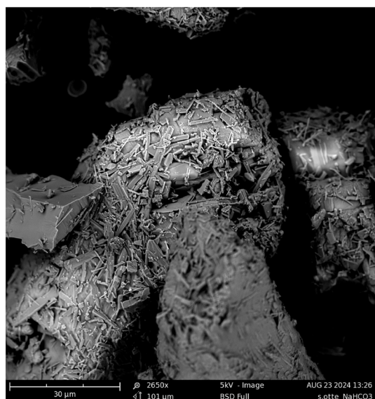
Figure 13. SEM image with 2650x magnification of sodium bicarbonate. The surface is unstructured and rough with individual rod-like structures.
