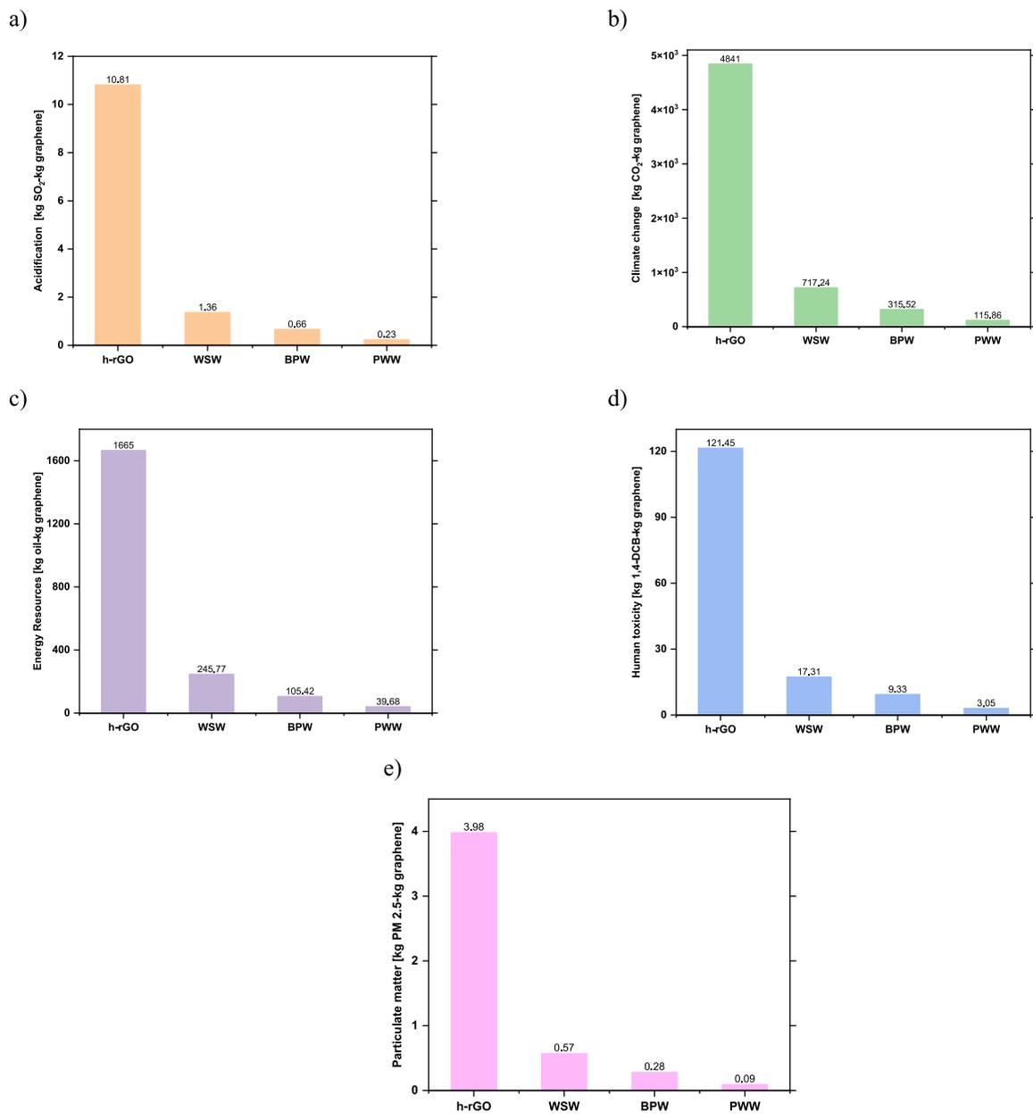
Fig. 2. LCIA results using the ReCiPe method. Values are presented per 1 kg of graphene production as the functional unit. a) acidification, b) climate change, c) energy resources, d) human toxicity, and e) particulate matter potential.
