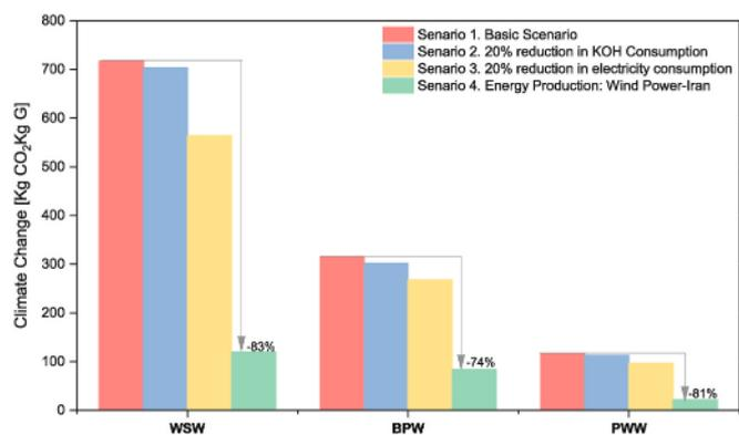
Fig. 6. Sensitivity analysis results for the GWP of biomass waste-derived graphene across all three precursors.
