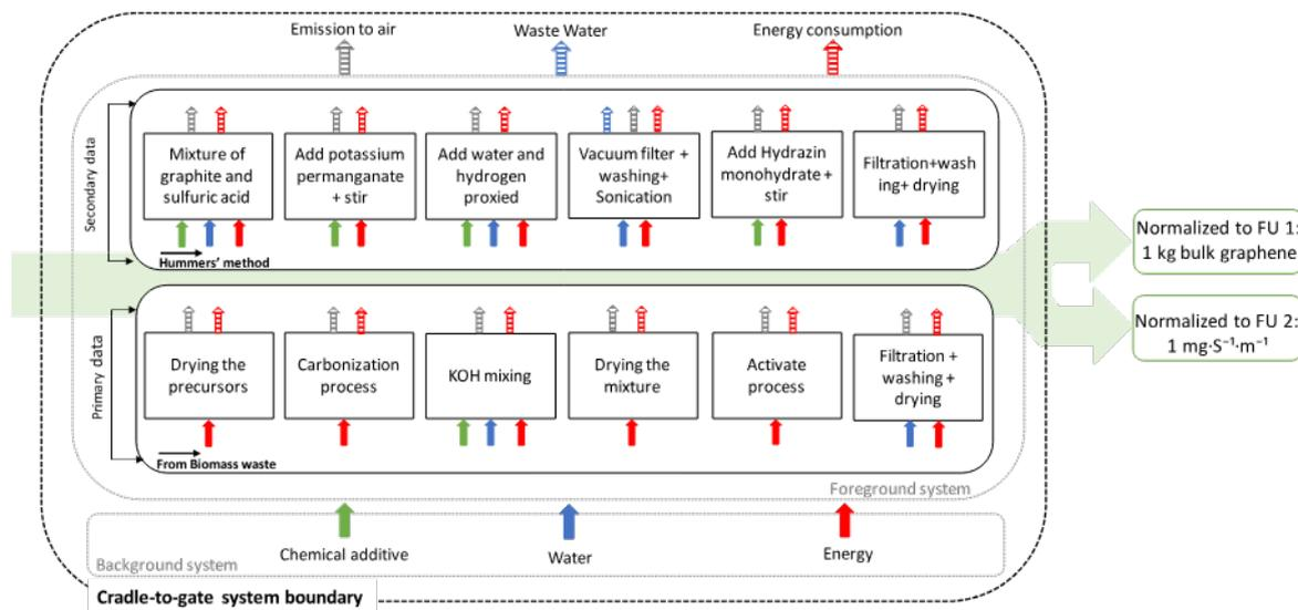
Fig. 1. Cradle-to-gate system boundary applied in the LCA methodology for Graphene Production from Biomass Waste and Hummers' Method (Serrano-Luján et al., 2019).
