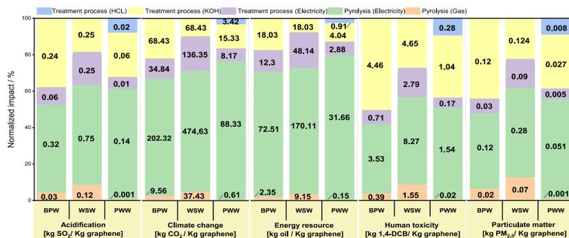
Fig. 3. Synthesis process contribution analysis of environmental impact for three precursors. The absolute values for each synthesis process contribution, expressed in units, are presented in the respective columns.
