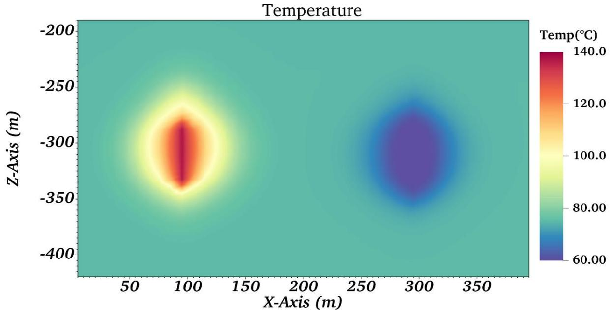
Figure 2: Variation of temperature at a hot and a cold well after 5 years of seasonal injection and production cycles.
