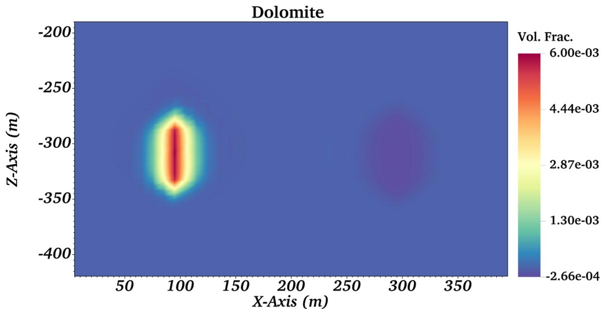
Figure 7: Dolomite changes (volume fraction) in the XZ-plane (Y=145 m) after 5 years of seasonal injection and production cycles.
