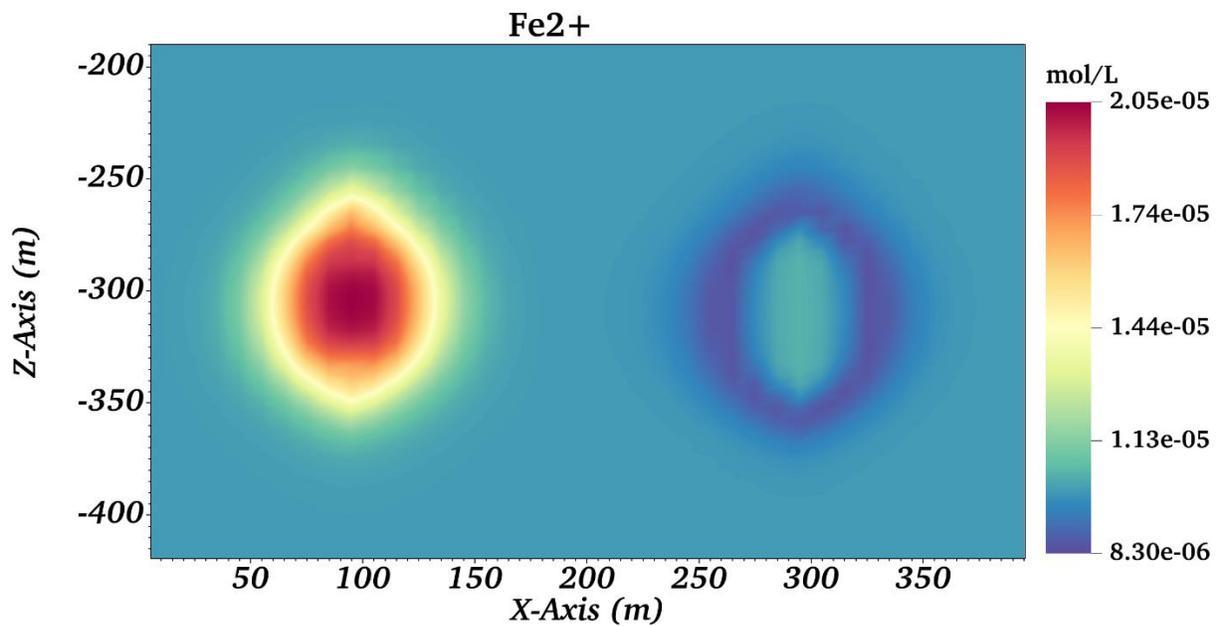
Figure 4: Concentration (mol/L) of  $\text{Fe}^{2+}$  in the XZ-plane (Y=145 m) after 5 years of seasonal injection and production cycles.
