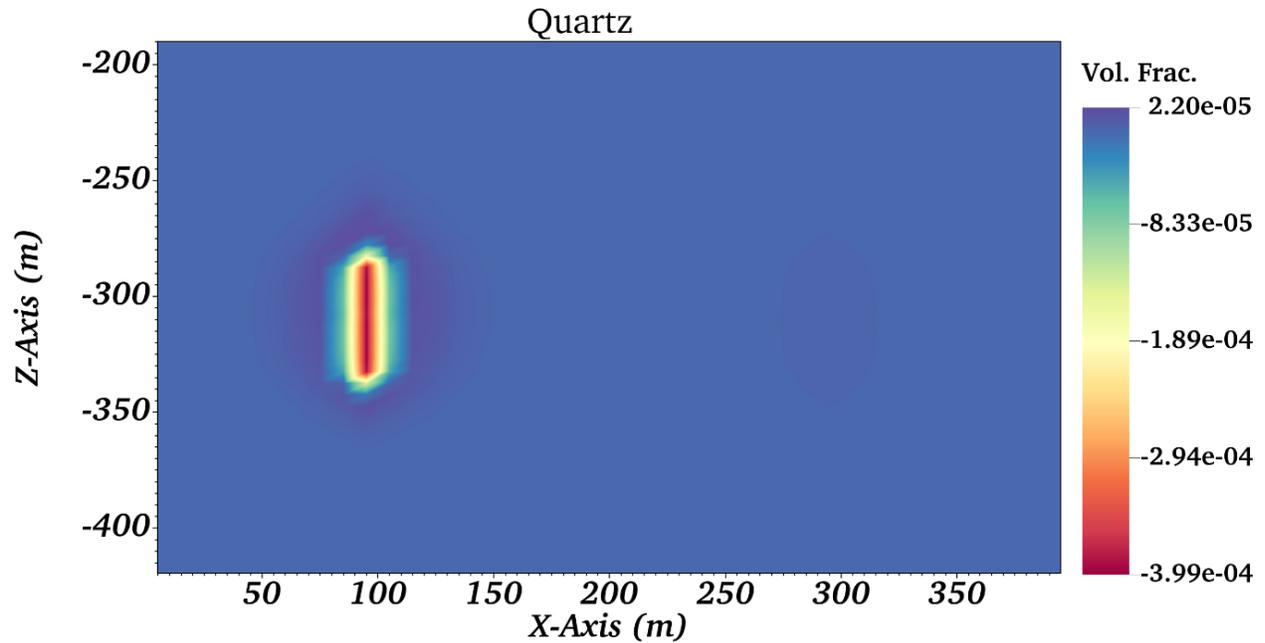
**Figure 8:** Changes in quartz (volume fraction) in the XZ-plane (Y=145 m) after 5 years of seasonal injection and production cycles.
