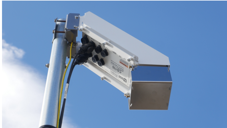
Figure 4.21: Picture of the zero-field cover mounted on the EFM at BATATA.
