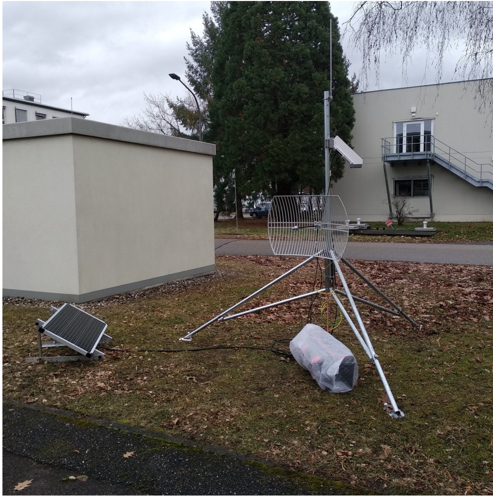
Figure 4.4: Test setup of a station for the new EFM network next to building 425 of IAP at KIT Campus North. On the right is a tripod with the EFM mounted on it and a lightning rod on top. The grid dish antenna points to a nearby office where the receiving system of sector antenna and rocket are placed and connected to the IAP network. In front of the tripod on the ground is a tool box wrapped in plastic foil holding all electronic components. On the left is a solar panel pointing south.
