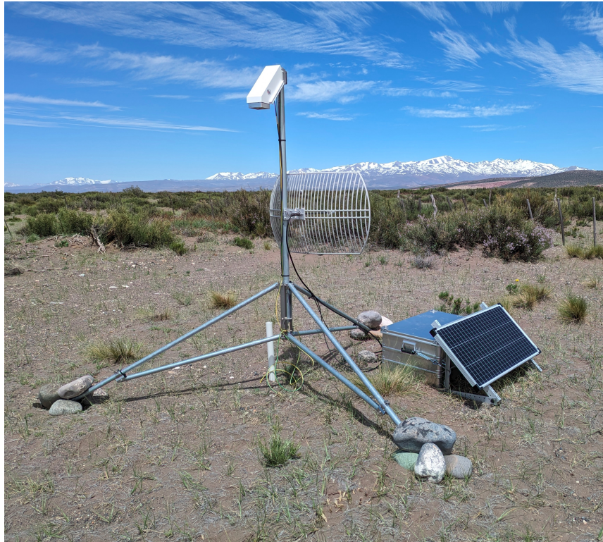
Figure 4.7: First deployed station guanaCO at the BATATA site with the existing fence in the background.
