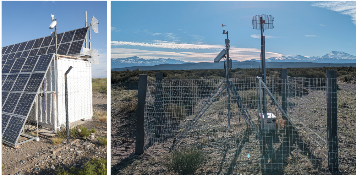
(a) EFM mounted on top of the western edge of the CRS container together with multiple other weather sensors. (b) EFM mounted in the field at the AERAWS station, also accompanied by other weather sensors.
