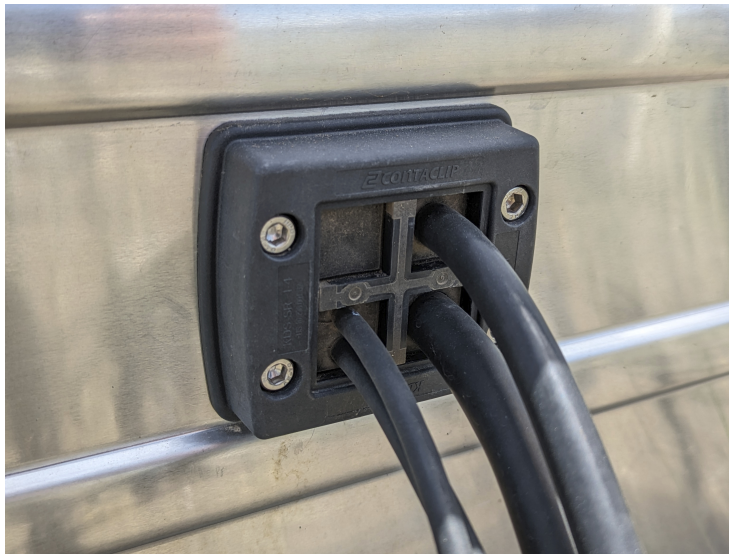
Figure A.1: Picture of the outside of an electronics box showing the cable glands.
