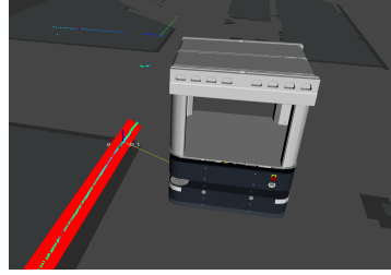
(b) Laser-based pose estimation of the docking pose associated with the transfer unit, see (Zhou et al. 2023).
