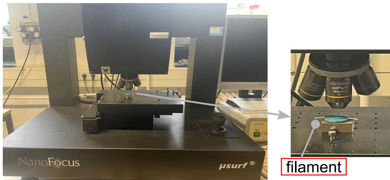
Figure 5. Left: procedure for surface roughness measurement by nanofocus; right: magnified view of the left figure.
