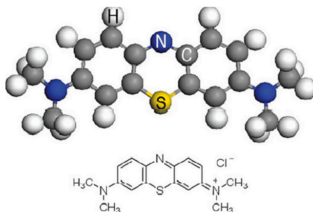
Fig. 1. Structure and model of MB dye molecule [41] (adapted with permission from the Royal Society of Chemistry, license ID 1079849–1).
