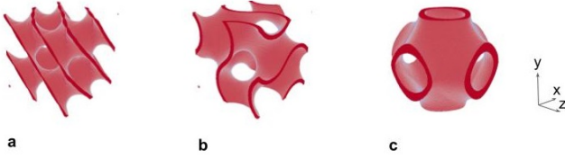
Figure 1.1: Examples of TPMS unit cells: a. Diamond; b. Gyroid; c. Primitive [3]
