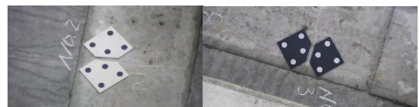
Figure 5. Targets placed on the bridge girder, captured using the SUNBA PTZ camera.
