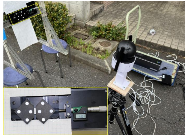
Figure 4. Laboratory set up of ANAKK at 1m from the micrometre (inset).
