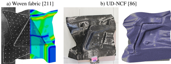
Figure 2.19: Examples for a continuous approach for a) a woven fabric and b) a UD-NCF.
