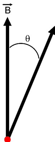
Figure 162. Rotational axis (red dot, oriented into the paper plane) and direction of B field with \theta being the angle the sample was rotated from the origin (aligned with B ).
