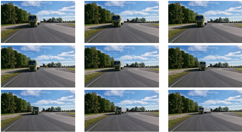
Figure 5.6.: Positive initial deviation with PPC-LC. The trailer starts in the fourth lane while the reference is in the third lane. The trailer fails to converge to the reference lane, indicating that the PPC-LC could not bring the system back to the desired trajectory.
