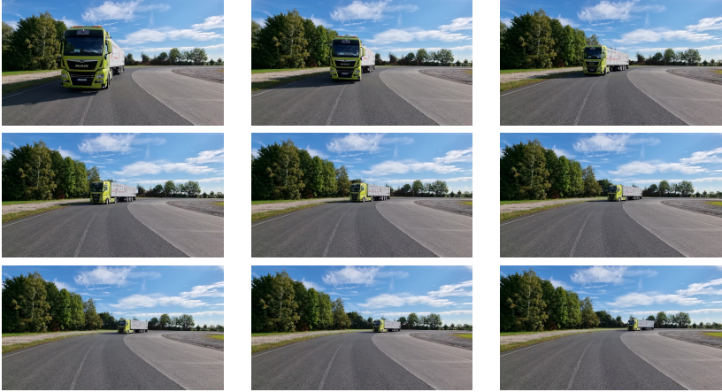
Figure 5.7.: Positive initial deviation with FMPC. The trailer starts in the fourth lane while the reference is in the third lane. The trailer successfully converges to the third lane, showing the effectiveness of the FMPC in correcting the trajectory.
