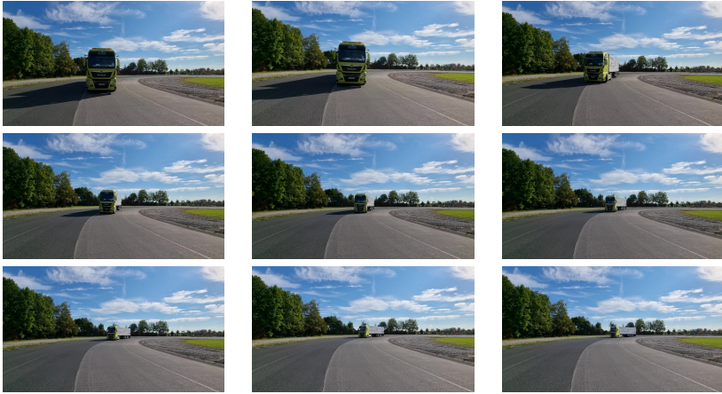
Figure 5.5.: Negative initial deviation with FMPC. The trailer starts in the second lane from the left while the reference is in the third lane in a circular path. The trailer successfully converges to the third lane without driver intervention.
