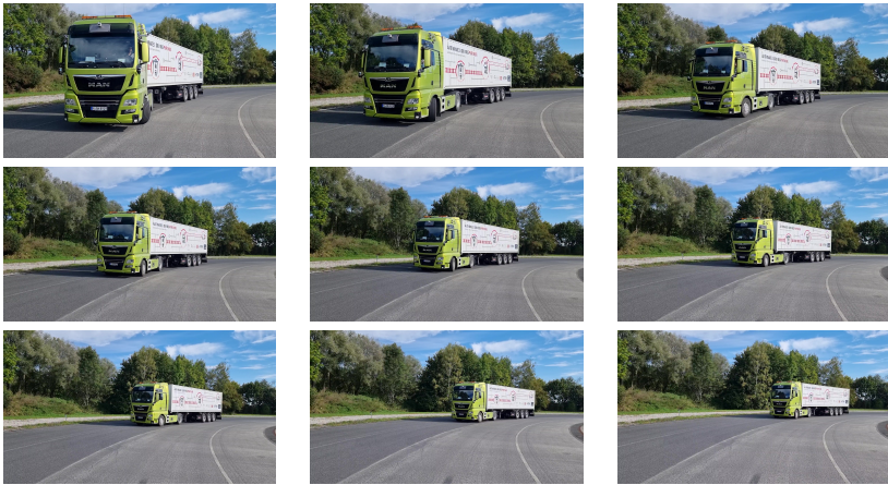
Figure 5.9.: FMPC with negative angle deviation. The trailer starts in the third lane with a slight misalignment at the start position. The system successfully converges to the desired trajectory.
