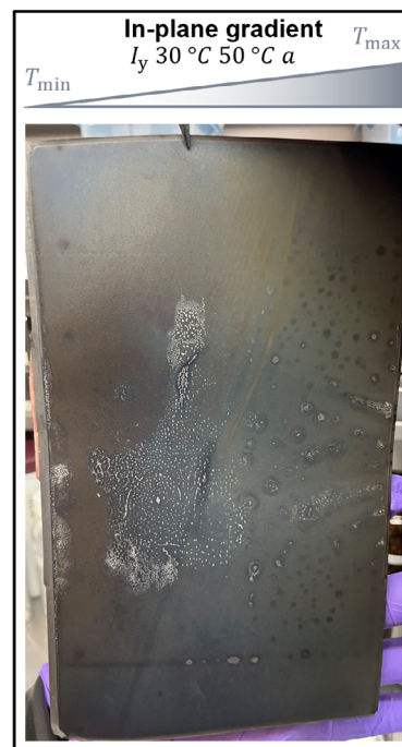
Figure 6. Negative electrode sheet from cell ( I_y 30 °C 50 °C a) aged with an applied in-plane thermal gradient from 30 to 50 °C.
