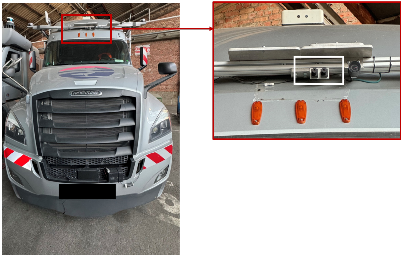
Figure 56: Position of two Leopard cameras above windshield on the truck
