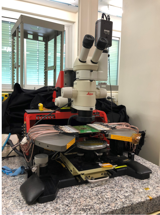
Figure 3.5: Wafer probe station with a probe card and a thermal chuck used to perform the back-bias measurements.
