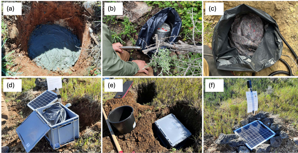
Figure 4. Installation of instruments of the 1A network in spring 2024: (a) Foundation for better surface coupling, (b) seismometer packed into bags, (c) thermal insulation, (d) equipment box, (e) two separated holes for equipment and seismometer, (f) final appearance of station MM09 with solar panel and warning sign at the GPS post.
