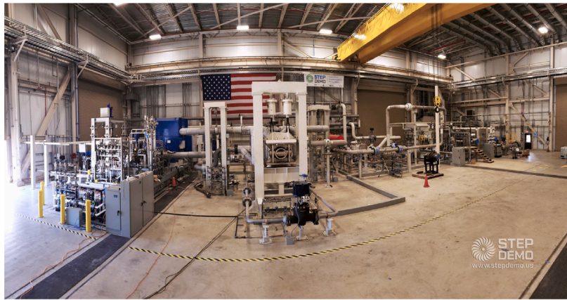
Fig. 4. 10 MW Supercritical Transformational Electric Power (STEP) Demo pilot plant by Southwest Research Institute (SwRI), figure from press release , used for educational and informational purposes.
