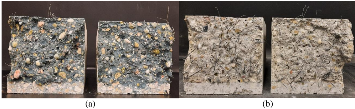
Figure 4: Example of broken tested beams for the mixes (a) AASC-3D75 and (b) PCC-3D75 used to count the number of fibres at the cross-section
