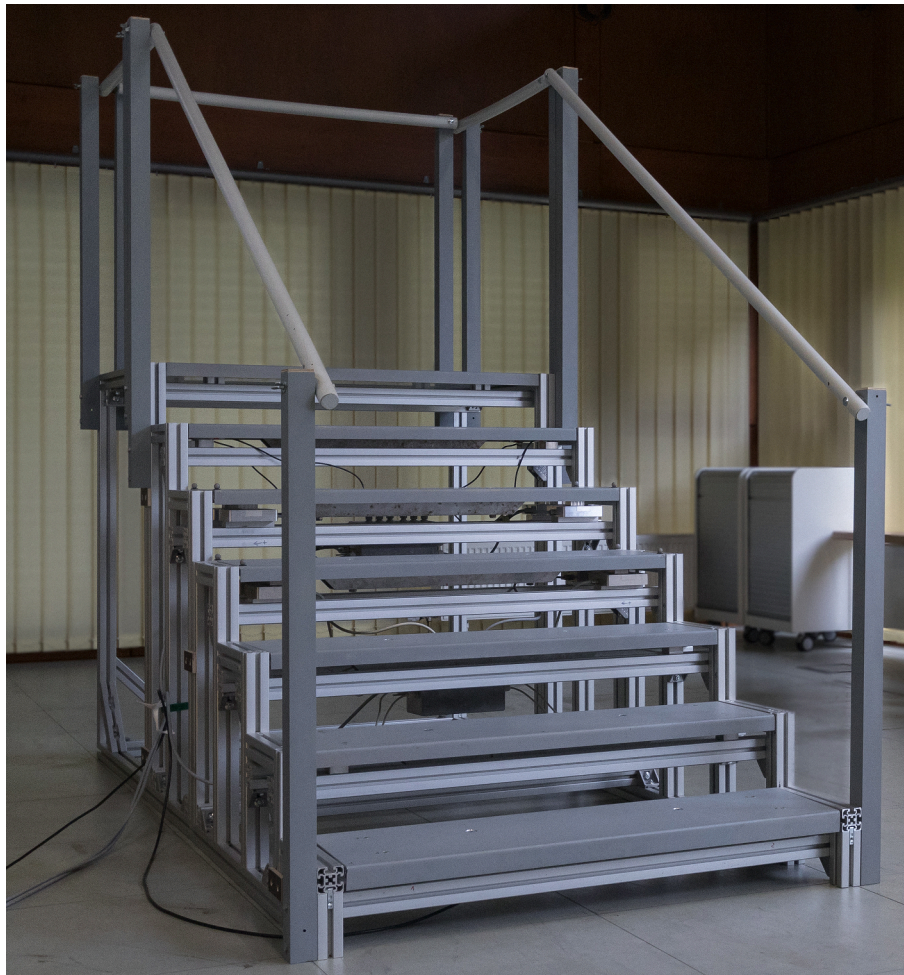
Fig. 1. Picture of the instrumented staircase. Three-dimensional force plates in steps four and five from the bottom, one-dimensional force plates in steps one to three and six. Riser height = 17 cm, tread = 28 cm, inclination angle = 31.26°.
