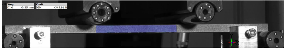
Fig. 3 Screenshot of the ARAMIS definition for the bending test of the first load cycle. The area of evaluation was chosen such that it is located within the inner supports. Also visible are the supports used and the aligners, which are coated with Teflon on the inside
