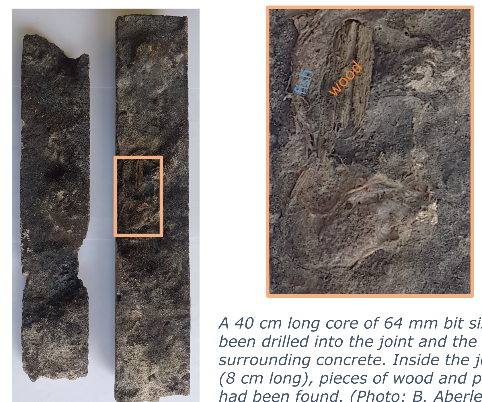
Part of a 40 m long open construction joint found at km 13.7 in the pressure tunnel. In this tunnel section, mud, larger fish and pieces of wood and plastic got stuck (Photo B. Aberle).
