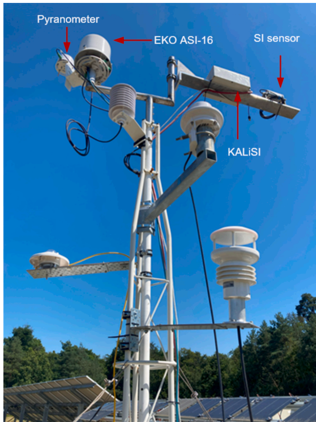
Fig. 2. Photograph showing the KALiSI mounted on the weather station mast at the KIT Solar Park. The EKO ASI-16 commercial sky imager can also be seen, along with the SI sensor for measuring GHI (for KALiSI) and the dedicated pyranometer (EKO Instruments, MS80HS, Japan) for the EKO sky imager. Several sensors that are not utilised in this work are mounted below the sky imagers: a precipitation sensor (Lufft, WS100, radar sensor, Germany) an additional pyranometer (Kipp & Zonen, SMP12, The Netherlands), and a multi-weather sensor (Thies Clima sensor US, NHTFB, Germany).
